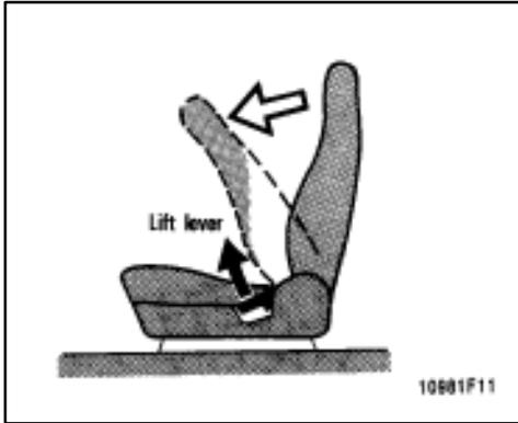
**Lift seatback lock release lever—the seatback will tilt forward.**
