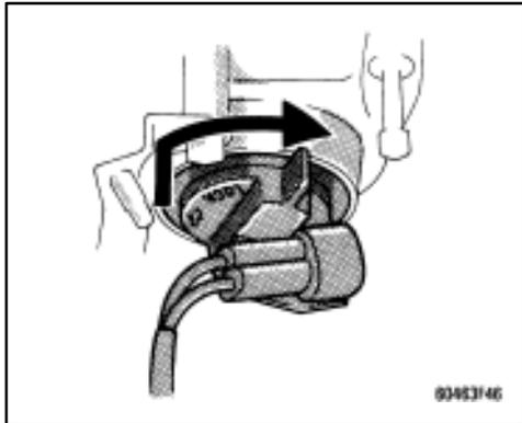
**5. Connect the cords and install the cover by turning it clockwise.**
