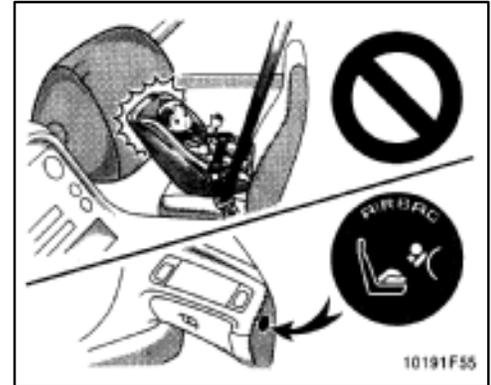
ⓈNever put a rear-facing child restraint system in the front seat because the force of the rapid inflation of the passenger airbag can cause severe injury to the child. Vehicles with a passenger airbag display a caution label on the passenger side instrument panel as shown above to remind you not to install a rear-facing child restraint system on the front seat.
