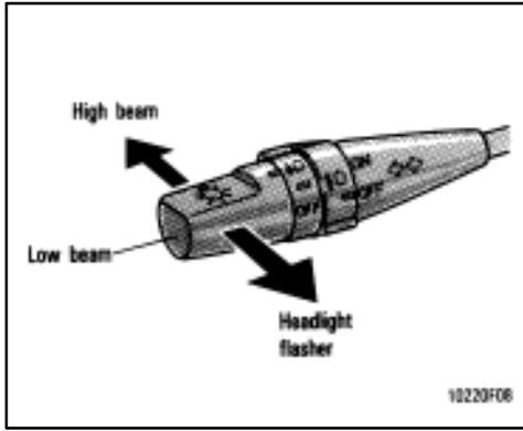
For high beam, push the lever away from you. Pull it toward you for low beam. For the headlight flasher, pull it further back.
