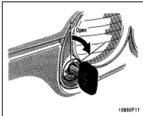
To open the back door from the outside, insert the key and turn it clockwise.
