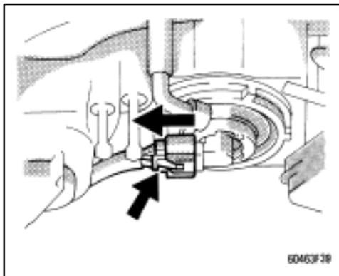
**2. Unplug the connector while depressing the lock release.**
