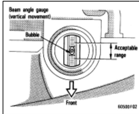
**To check the headlight aim, check the vertical and horizontal gauges.**
