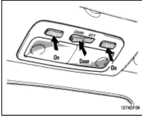
**To turn on the interior light, slide the switch.**
