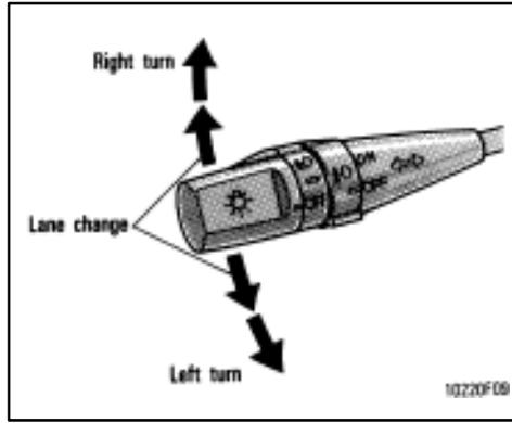
For signaling turns, move the lever up or down in the conventional manner.
