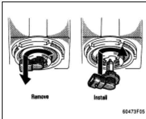
**3. Turn the bulb clockwise and remove it. Install a new bulb, turn it counterclockwise, then plug in the connector.**
