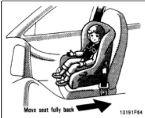
Ⓜ If you must use a forward-facing child restraint system in the front seat, the seat must be moved as far back as possible. For instructions concerning the installation of a child restraint system, see “Child restraint” in this chapter.
