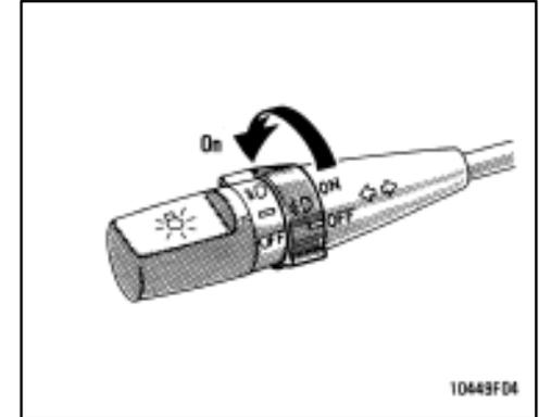
To turn on the front fog lights, twist the knob of the headlight and turn signal switch lever. They will come on when the headlights are turned on low beam.
