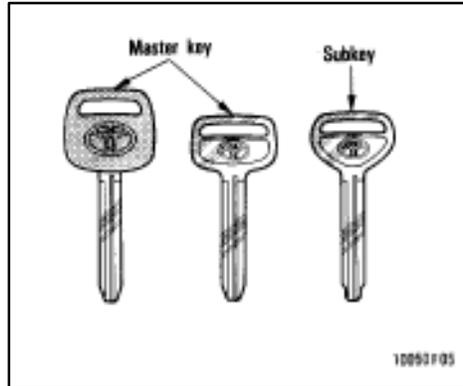
**The master key works in every lock. The subkey will not work in the glovebox.**
