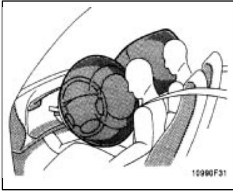
The SRS (Supplemental Restraint System) airbags are designed to provide further protection to the driver and front passenger when added to the primary protection provided by the seat belts.
