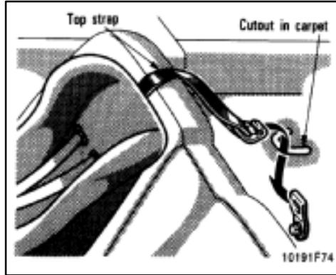
**If your child restraint system requires the use of a top strap, latch the hood onto the anchor bracket and tighten the top strap.**
