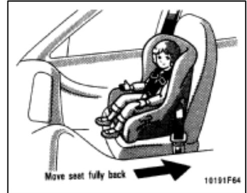
Ⓢ Only when it is unavoidable should a forward-facing child restraint system be used on the front seat. Always move the seat as far back as possible because the force of deploying airbag would cause serious injury to the child.
