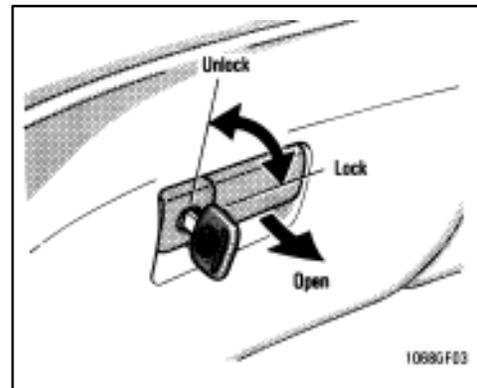
**To open the glovebox door, pull the lever. To lock the glovebox door, insert the master key and turn it clockwise.**
