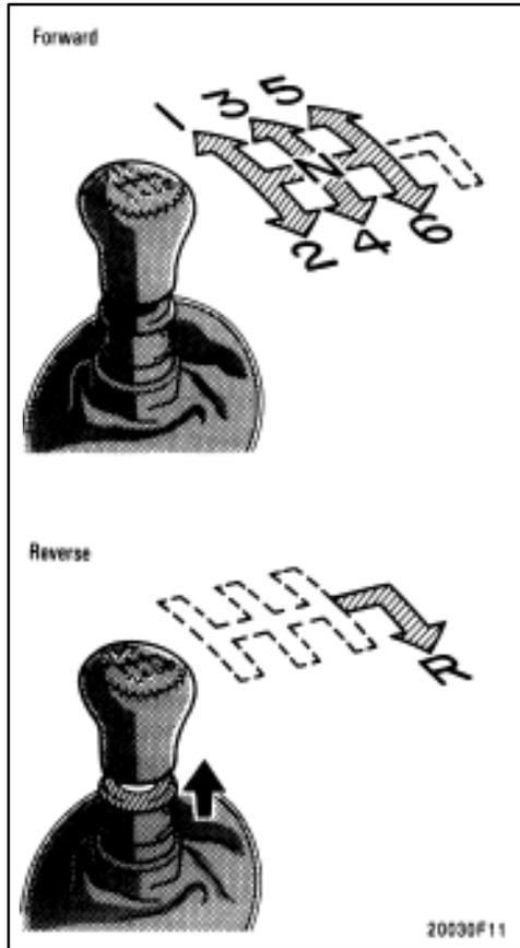
The shift pattern is shown above. You must lift up the ring around the gear shift lever to shift into “R” (reverse).
