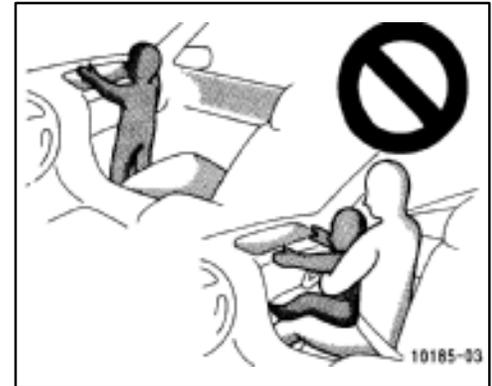
Ⓜ Do not allow a child to stand up, or to kneel on the front passenger seat. The airbag inflates with considerable speed and force; the child may be severely injured.
