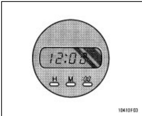
Once the electrical power source has been disconnected from the clock, the time is automatically set to 1:00 (one o'clock).
