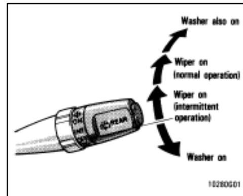
To turn the rear wiper and washer on, twist the knob at the end of the lever.
