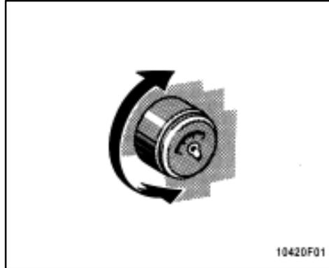
To adjust the brightness of the instrument panel lights, turn the knob.
