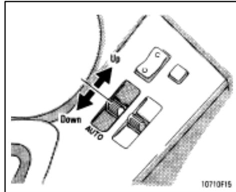
The windows can be operated with the switch on each side door.
