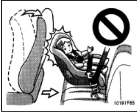
ⓈDo not use a rear-facing child restraint system in the rear seat if it interferes with the lock mechanism of the front seats. This can cause severe injury to the child and front passenger in case of sudden braking or a collision.
