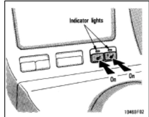
**To turn on the seat heater, push the "L" switch for the driver's seat, and "R" switch for the passenger's seat.**
