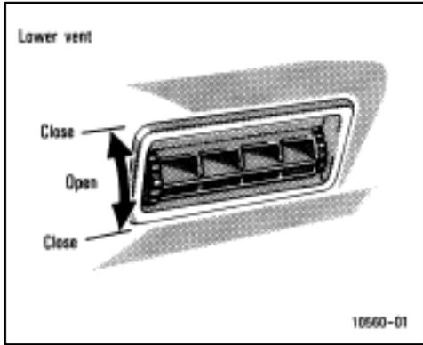
If air flow control is not satisfactory, check the instrument panel vents. The instrument panel vents may be opened or closed as shown.
