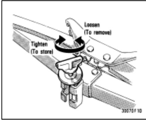
To remove the jack, loosen the bolt and remove it.
