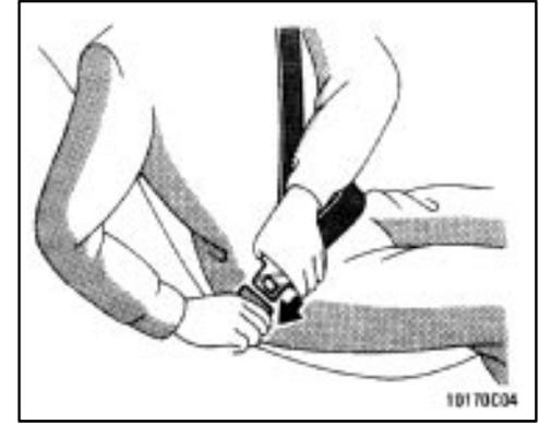
Adjust the seat as needed (front seats only) and sit up straight and well back into the seat. To fasten your belt, pull it out of the retractor and insert the tab into the buckle.
