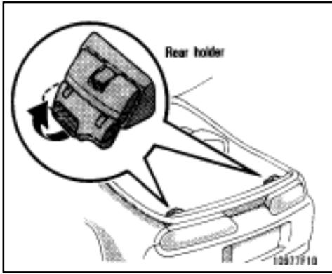
1. Open the back door and set up the rear holders as shown above.
