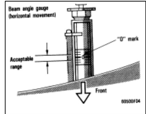
2. Look at the beam angle gauge (horizontal movement). The "0" mark should not deviate by more than one mark on either side of the gauge.
