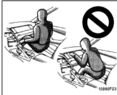
Ⓜ Do not sit on the edge of the seat or lean over the dashboard when the vehicle is in use. The airbags inflate with considerable speed and force; you may be severely injured. Sit up straight and well back in the seat, and always use your seat belt.
