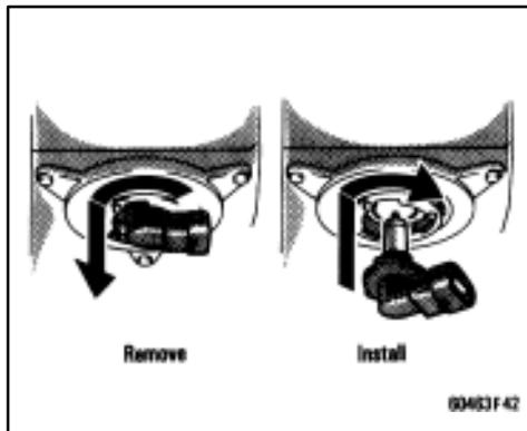
**3. Turn the bulb counterclockwise and remove it. Install a new bulb, turn it clockwise, then plug in the connector.**
