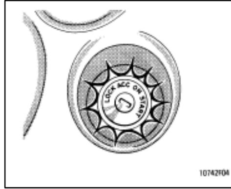
**For easy access to the ignition switch, the ignition switch light comes on when either side door is opened.**
